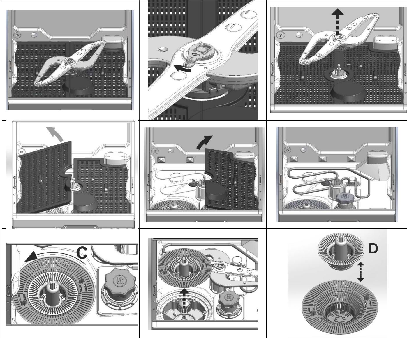
**Procedure to disassemble the filters made of 2 filtering elements:
