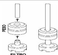
Before inserting the hoses into the containers, fit the weights (needed to ensure that they always draw in liquid from the bottoms of the containers) and the filters onto their ends as shown. If the detergent dispenser is not factory-fitted, it can be retrofitted after ordering the relative kit.
